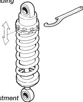
Mechanical pre-loading adjustment
